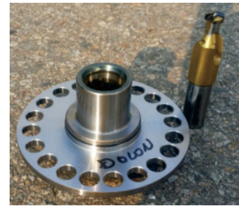
After drilling & back chamfering
