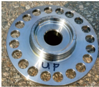
After drilling & front chamfering
