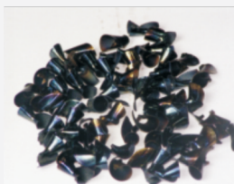
Chip feature after drilling
